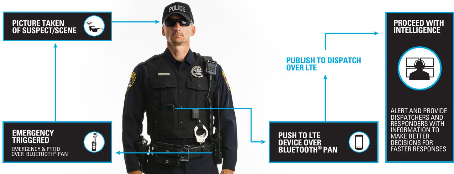
An officer pushes the emergency button on his P25 digital LMR radio, which automatically notifies dispatch and triggers his wearable camera to take a photo of the suspect and the scene. The push-to-talk ID (PTTID) and the photo are sent to dispatch via the officer's Bluetooth® Personal Area Network (PAN) over the LTE network. Dispatch pushes the officer information, location and photo to nearby units who quickly arrive on the scene to provide assistance.
